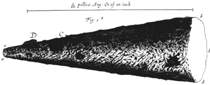
But if viewed with a very good *Microscope*, we may find that the *top* of a Needle (though as to the sense very *sharp*) appears a *broad, blunt, and very irregular* end; not resembling a Cone, as is imagined, but only a piece of a tapering body, with a great part of the top removed, or deficient ...
